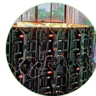
Modular curved enclosure design, easily creating immersive curved displays
